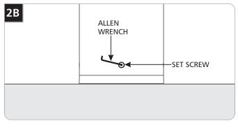
**5** Carefully install the fixture onto the base plate and secure it in place by tightening all set screws.
